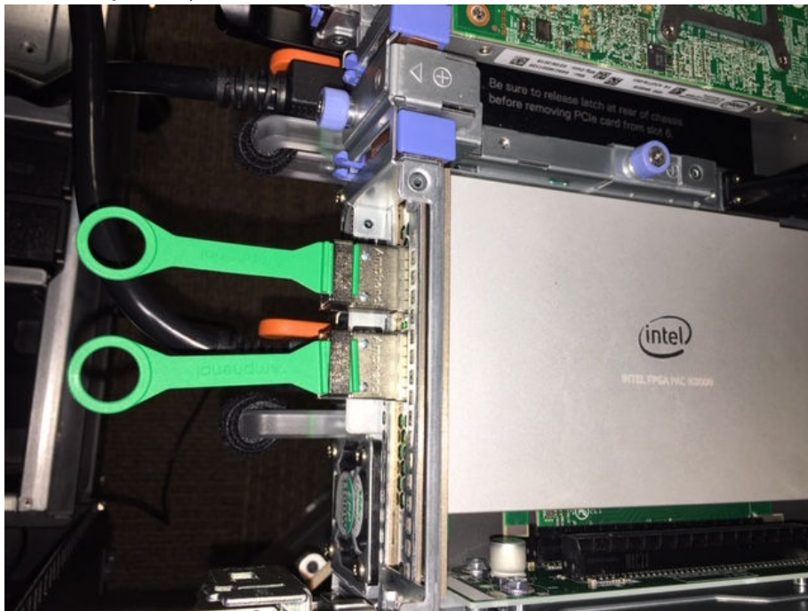
Figure 3. Example of QSFP Non-optical Modules
